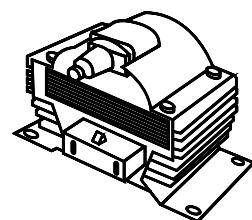
BluePrint recommends using a canister type coil when a Holley Sniper EFI is installed.
